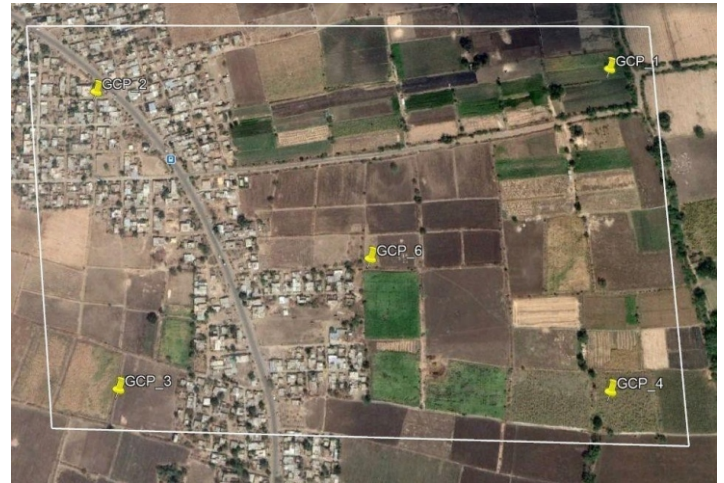
Figure: Drone AOI with GCP placement
