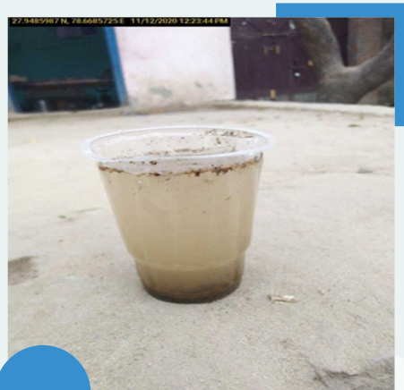
Turbid due to suspended material UP_DHARAMPUR 1_111771_029241_W1
