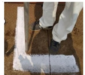
Figure: Sample GCP, placement on ground and taking reading on it
