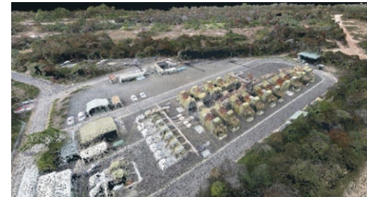
Figure: Point Cloud processed from Images
