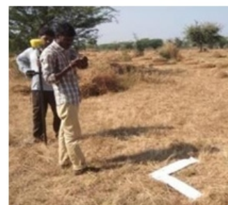
Figure: Sample GCP, placement on ground and taking reading on it
